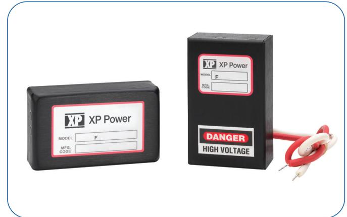
The F Series is a broad line of robust, field-proven DC to HV DC converters which deliver 10 Watts continuous output power. Outputs range from 100V to 12kV. The input and output are galvanically isolated so a unit can be used to deliver a positive or negative high voltage output. The output voltage is proportional to input voltage with a low 0.7V typical turn-on voltage.
