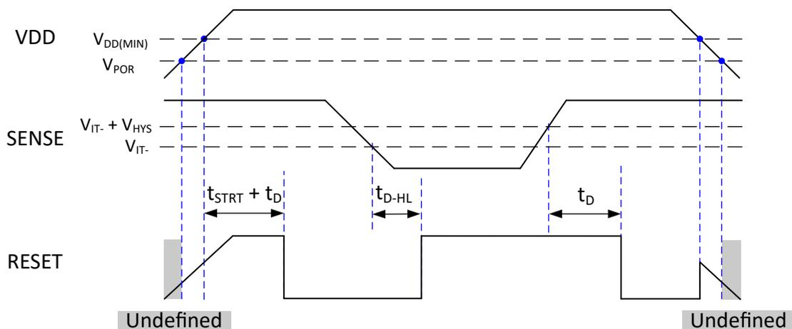
A. Open-Drain timing diagram assumes the RESET pin is connected via an external pull-up resistor to VDD.
