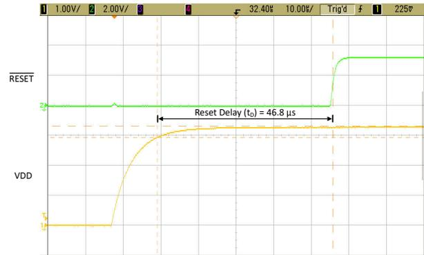
Figure 9-4. TLV841EVM  $\overline{\text{RESET}}$  Time Delay ( $t_D$ )
