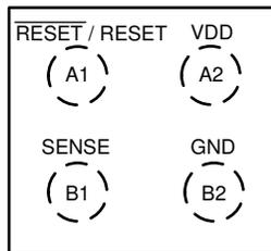
**Figure 6-1. YBH 4-Pin DSBGA Package (TLV841S) Top View**
