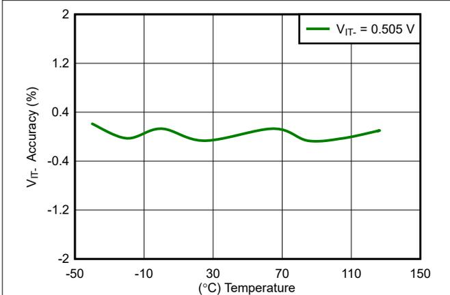
**Figure 7-7.  $V_{\text{IT-}}$  Accuracy vs Temperature**
