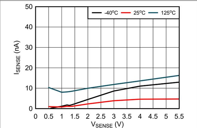
**Figure 7-6. SENSE Current vs  $V_{\text{SENSE}}$**
