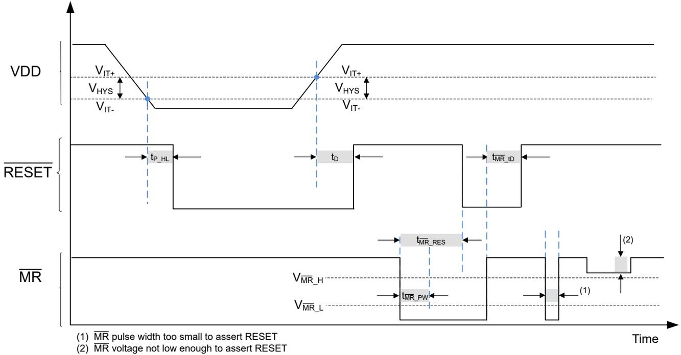
**Figure 8-6. Timing Diagram  $\overline{\text{MR}}$  and  $\overline{\text{RESET}}$  (TLV841M)**
