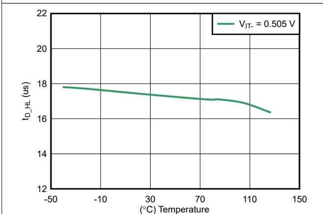
**Figure 7-9. SENSE Delay ( $t_{D\_HL}$ ) vs Temperature**
