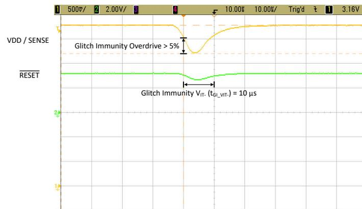
Figure 9-5. TLV841EVM SENSE Pin Glitch Immunity ( $t_{GI\_VIT-}$ )
