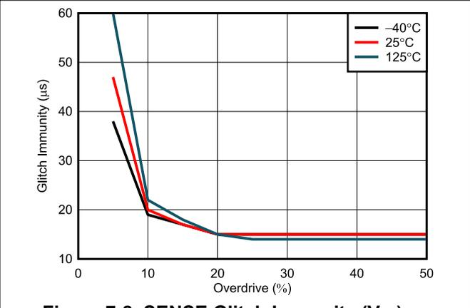
**Figure 7-8. SENSE Glitch Immunity ( $V_{\text{IT-}}$ ) vs Overdrive**
