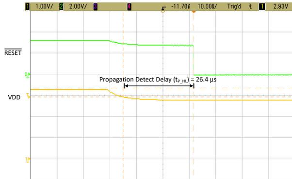
Figure 9-3. TLV841EVM Propagation Delay Time Delay ( $t_{D\_HL}$ )
