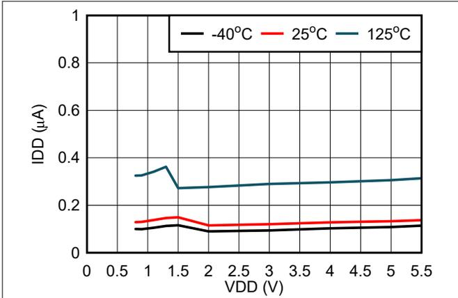
**Figure 7-5. Supply Current vs Supply Voltage for TLV841S**
