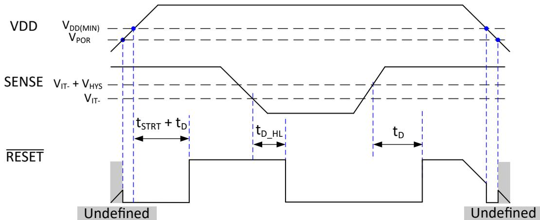
A. Open-Drain timing diagram assumes the  $\overline{\text{RESET}}$  pin is connected via an external pull-up resistor to VDD.
