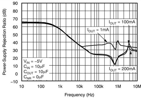
Figure 25. PSRR vs Frequency
