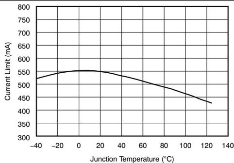
Figure 9. TPS72325 Current Limit vs Junction Temperature
