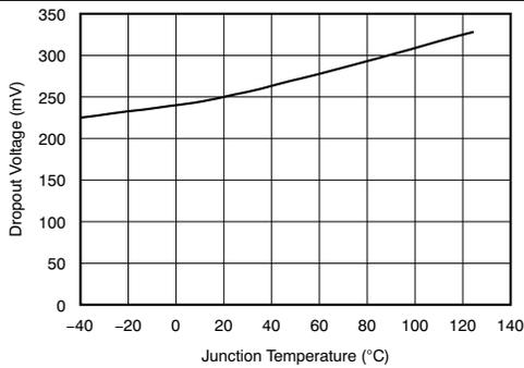
Figure 5. TPS72325 Dropout Voltage vs Junction Temperature
