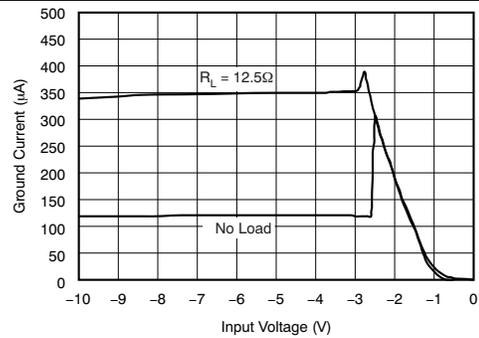
Figure 6. Ground Current vs Input Voltage
