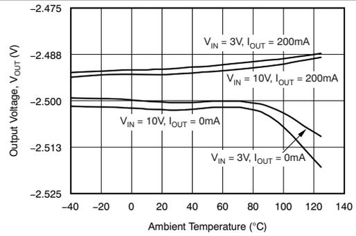
Figure 2. Output Voltage vs Ambient Temperature
