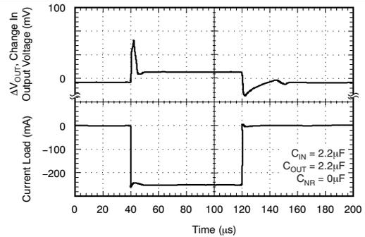
Figure 16. TPS72325 Load Transient Response
