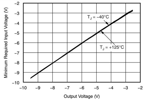
Figure 14. TPS72301 Minimum Required Input Voltage vs Output Voltage
