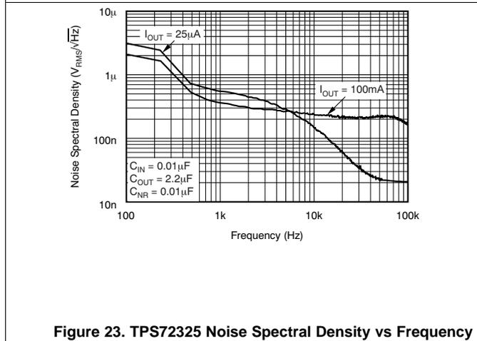
Figure 23. TPS72325 Noise Spectral Density vs Frequency
