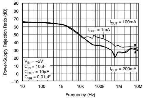
Figure 26. PSRR vs Frequency
