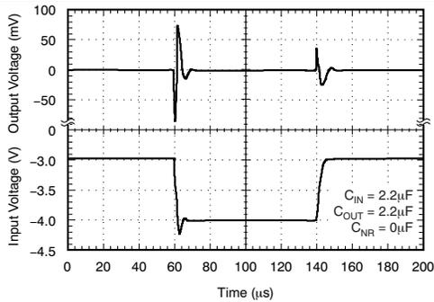
Figure 15. TPS72325 Line Transient Response
