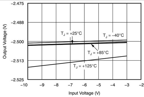
Figure 1. Output Voltage vs Input Voltage
