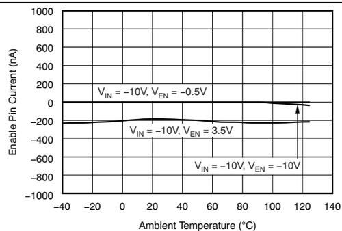
Figure 12. Enable Pin Current vs Junction Temperature
