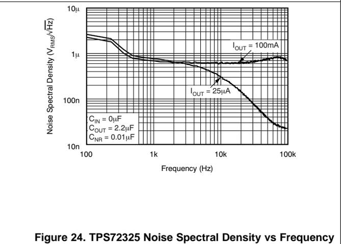
Figure 24. TPS72325 Noise Spectral Density vs Frequency
