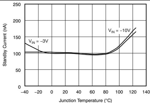
Figure 10. Standby Current vs Junction Temperature
