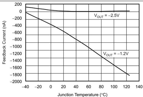
Figure 11. TPS72301 Feedback Pin Current vs Junction Temperature
