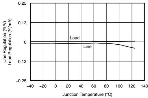
Figure 13. Line And Load Regulation vs Junction Temperature
