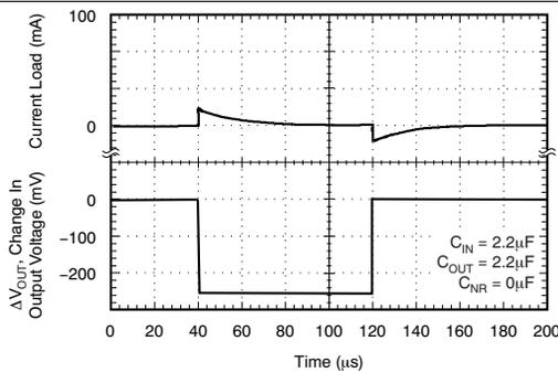
Figure 17. TPS72325 Load Transient Response
