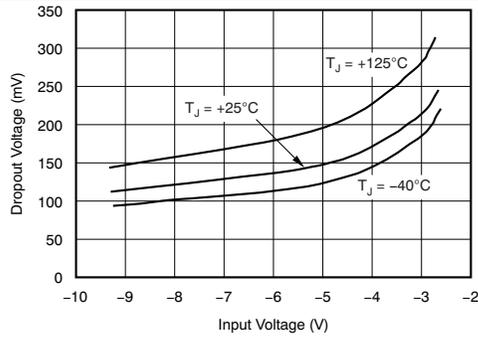
Figure 3. TPS72301 Dropout Voltage vs Input Voltage
